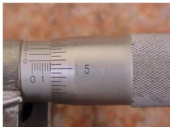
8.) The O.D. Micrometer on the Left is reading:
