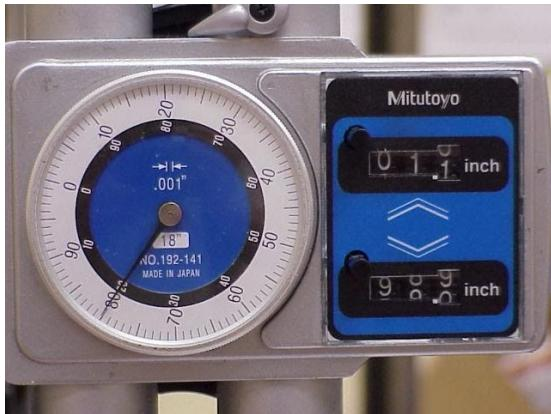
10.) The Height Gage on the Left is reading in the upward position:
