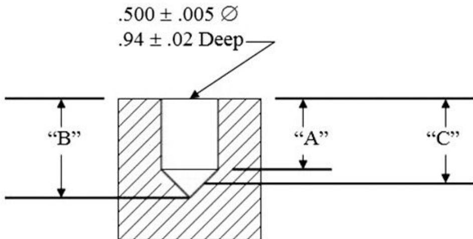
18). The depth of a tapped hole that is drilled into a cast surface, which is considered draft angle, is measured from:
