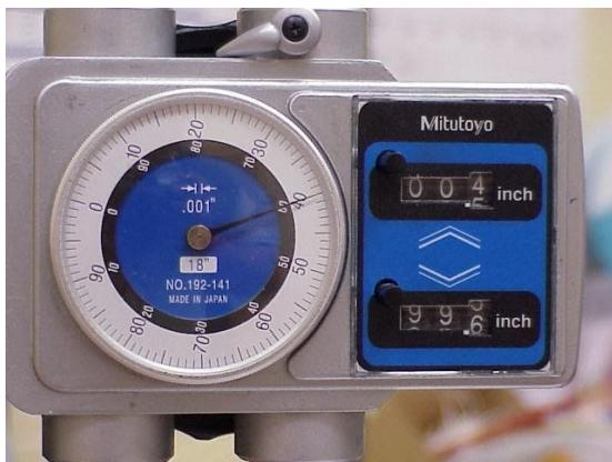
12.) The Height Gage on the Left is reading in the upward position:
