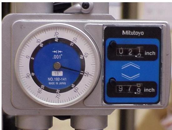
11.) The Height Gage on the Left is reading in the upward position:
